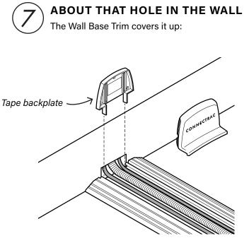
Use mounting tape to stick the backplate against the wall base, making sure to align the legs in the aluminum bottom track. Use screws for additional support.
