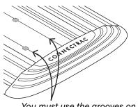
You <u>must</u> use the grooves on either side of the bottom track to stagger screws
