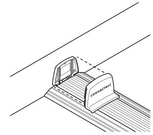
Set aside the frontplate until after the top cap is installed, then snap the frontplate onto the backplate.
