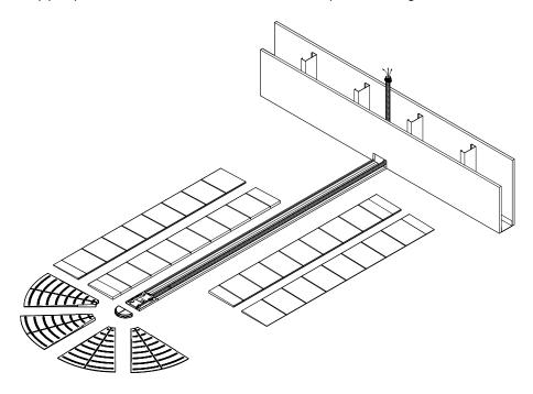
Secure the ramps to the floor slab with  $1/4" \times 11/4"$  pin-drive anchors.
