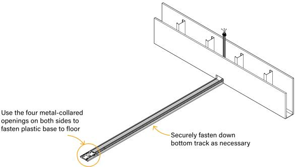
\*Raceway Extensions are placed at the end of the base Express Kit, before moving to step 5
